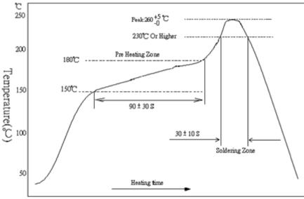
Remark: The peak temperature of soldering heat is 260 +5/-0  $^\circ\!{\rm C}$  for 10 seconds
